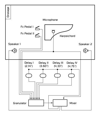
The granulator takes as input the main source and delayed lines granulating them with a density range from 0 to 100 grains per second; duration of grains should vary from 0.100 to 0.500 msec.
